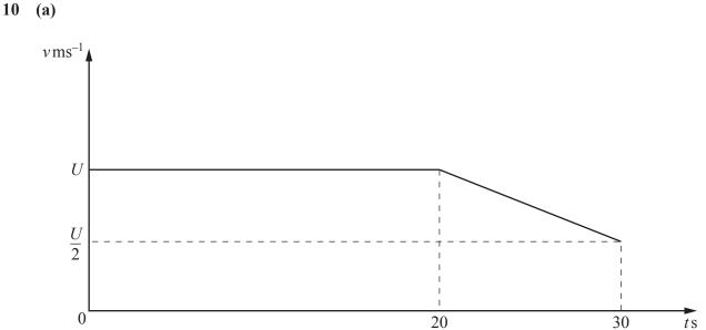
The diagram shows part of the velocity-time graph for a particle, moving at  $v \,\mathrm{ms}^{-1}$  in a straight line, *t*'s after passing through a fixed point. The particle travels at  $U \,\mathrm{ms}^{-1}$  for 20's and then decelerates uniformly for 10's to a velocity of  $\frac{U}{2} \,\mathrm{ms}^{-1}$ . In this 30's interval, the particle travels 165 m.
